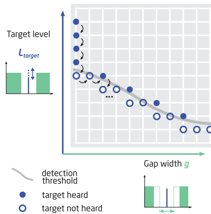
Fig. 1: Illustration of one run of the grid method. The track starts with a moderately high target level at zero gap width. Level is decreased until threshold is reached, after which gap is increased until the target can be heard again.
