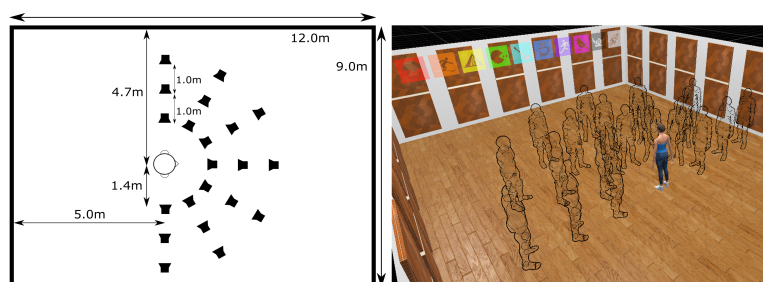
Fig. 1: (Left) Overview of the acoustic scene setup. The room was 2.8m high. The 21 simulated talker positions are indicated by loudspeaker symbols. (Right) Overview of the visual scene setup visually. Semi-transparent humanoid bodies were positioned at locations corresponding to the acoustic source positions.
