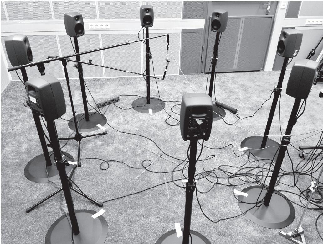
Fig. 1: The measurement setup consists of 8 loudspeakers, one reference microphone and one state-of-the-art hearing aid (BTE) connected to an ear simulator. The BTE is facing the loudspeaker in 0^\circ . Not shown is the RME fireface 800 soundcard and the PC.
