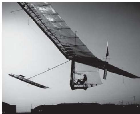
Fig. 3: The Gossamer Albatross, the first human-powered airplane that crossed the English channel. Figure from Raskin (2011).
