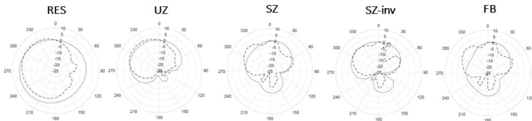
Fig. 1: Polar patterns of the five beamformer settings (left ear) calculated in octave bands with centre frequencies of 517 (low frequencies, solid line) and 1981 (high frequencies, dashed line). The azimuth is in degrees and the gain in dB.
