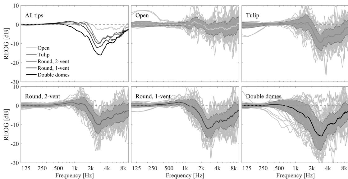
**Fig. 2:** Average REOG across 58 ears for the five ear tips (top left). The other panels show the average REOG per tip (thick line) and  $\pm$  1 standard deviation (shaded area). The light grey lines represent individual measurements.
