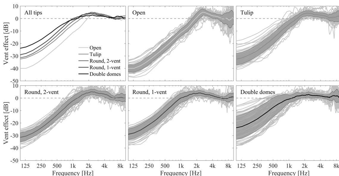
**Fig. 3:** VE, averaged across 58 ears for each ear tip (top left). The other panels show the average VE per tip (thick line) and  $\pm 1$  standard deviation (shaded area). The light grey lines represent individual measurements.
