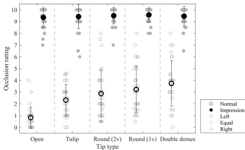
**Fig. 4:** Individual occlusion ratings (grey) and mean +/- one standard deviation (black). Circles indicate equal amounts of occlusion on both ears, triangles point in the direction of stronger occlusion.
