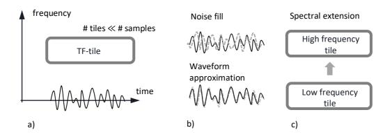
**Fig. 2:** Currently deployed audio coding tools. Panel a) shows the sharing of information in a TF-tile, panel b) the difference between waveform approximation and noise fill, and panel c) the principle of spectral extension.
