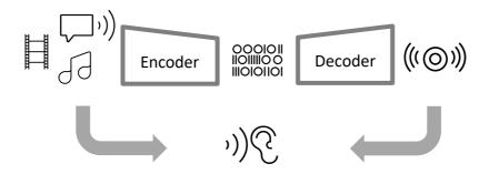
**Fig. 1:** Audio coding systems encode original sound sources into bits which can be transmitted and decoded into sound again at the receiver end. The combination of an encoder and decoder is called a *codec*.
