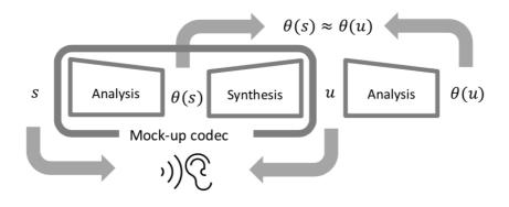
**Fig. 4:** Synthesis by analysis aims at producing a signal u given the analysis  $\theta(s)$  of an original signal s by solving  $\theta(u) \approx \theta(s)$ .
