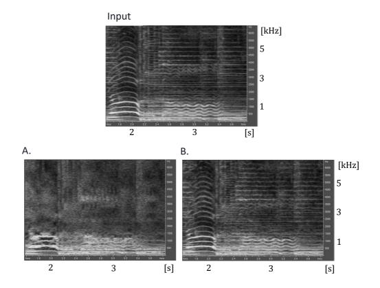
**Fig. 7:** Spectrograms of input and synthesis from (A) baseline and (B) extended representation for a segment of singing over guitar.
