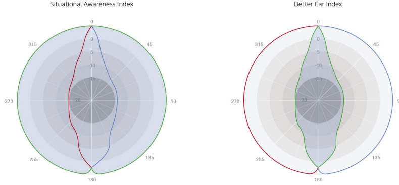
Fig. 3: Calculation of the metric. Left panel: Maximum power of across ears illustrates Situational Awareness Index (SAI). Right panel: Minimum power across ears (green line) illustrates Better-Ear Index. Grey shaded areas illustrate meaning of the indices.
