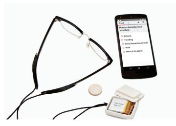
**Fig. 1:** Prototype of EMA system: Microphones attached to glasses, pocketsized Bluetooth transmitter, and smartphone with questionnaire
