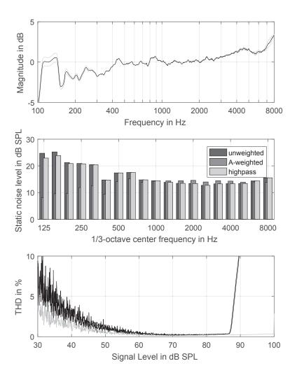
**Fig. 3:** *Top:* Frequency response of the current system, smoothed in ERB bands. Individual microphone responses are drawn as grey lines, the averaged response is drawn in black. *Middle:* Third-octave noise levels for different pre-processing filters. *Bottom:* Average percentage of total harmonic distortion by the system (black line) and reference microphone (grey line).
