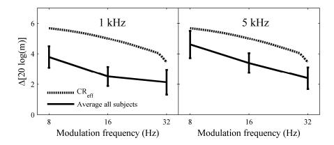
**Fig. 5:** The effect of WDRC on the modulation detection thresholds. The left panel is the result for the 1-kHz carrier and the right panel is the result for the 5-kHz carrier. For comparison, the black dotted curves display the physical reduction of the modulation depth from Fig. 2.
