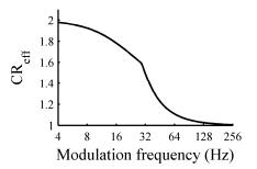
**Fig. 2:** The effective compression ratio ( $CR_{eff}$ ) for the used WDRC system as function of modulation frequency (e.g., Stone and Moore, 1992).
