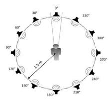
Fig. 5: Setup of the localization experiment.
