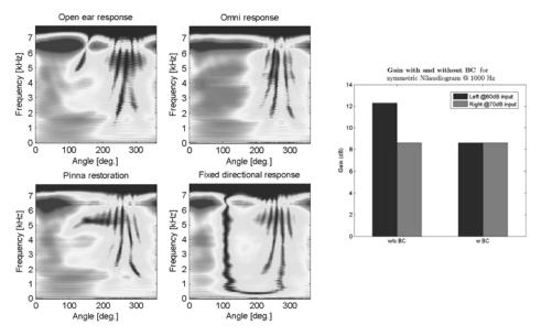
**Fig. 1:** Left panel: Intensity plots showing the open ear, omnidirectional, Pinna Restoration (PR) and Fixed Directionality (Dir) responses. The hearing aid was placed on KEMAR's left ear. Right panel: Gain, given with and without Bilateral Compression for a typical audiogram
