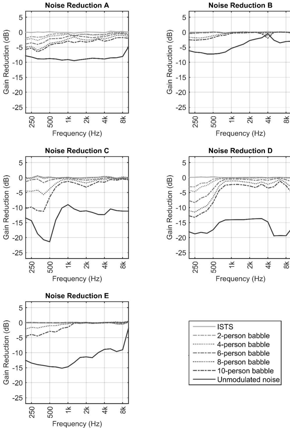
**Fig. 3:** Long-term average gain reduction in one-third octave bands for each of the seven test signals used. Every line represents the difference between noise reduction on and off averaged over 25 seconds after a 35-second pre-conditioning time.
