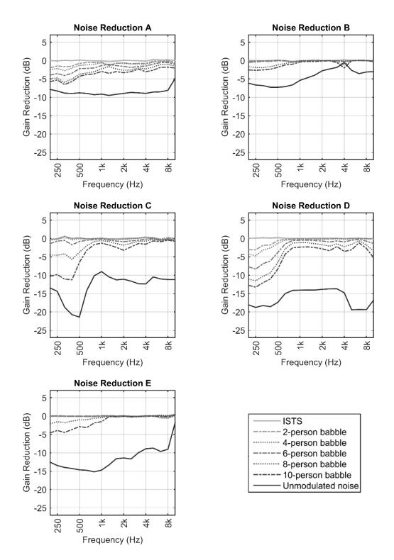
**Fig. 3:** Long-term average gain reduction in one-third octave bands for each of the seven test signals used. Every line represents the difference between noise reduction on and off averaged over 25 seconds after a 35-second preconditioning time.
