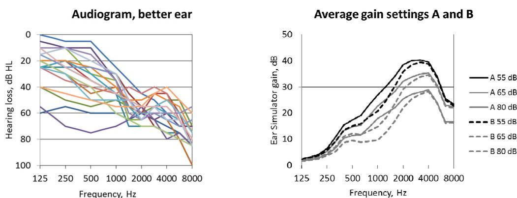
**Fig. 1:** Left: Better ear audiometric thresholds for all participants. Right: Average hearing-aid gain (Ear simulator) for the two prescriptions A and B measured using speech at three input levels (55, 65, and 80 dB SPL).
