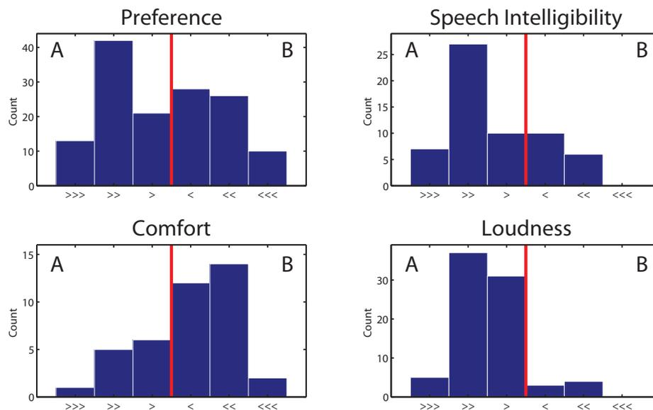
**Fig. 4:** Laboratory PC results for the attributes when all sound stimuli were pooled. Bars to the left of the vertical line indicate that A was selected more often, bars to the right that B was selected more often. The y-axes represent the total number of ratings. The symbols on the x-axes indicate the magnitude of difference between the two programs.
