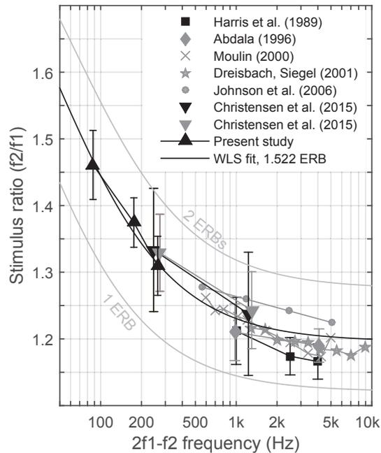
**Fig. 4:** Optimal ratios for DPOAE measurements as found by seven independent studies, including the present one (full references given in Christensen *et al.* (2015a)). The results comprise measurements in 98 individual subjects. Shown also is the least-squares fit of the ERB model to the data sets, weighted by the number of subjects they each represent.
