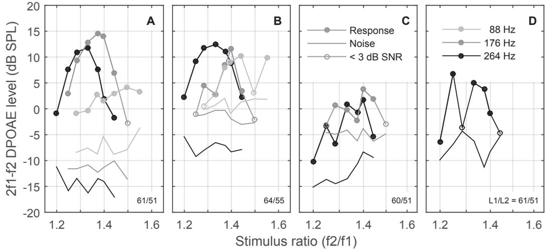
**Fig. 2:** Individual DPOAE levels as a function of the stimulus ratio  $f_2/f_1$  at three different  $2f_1 - f_2$  frequencies. Data points with signal-to-noise ratios less than 3 dB were rejected and the entire curve was excluded from the average if more than three points were rejected.
