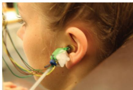
**Fig. 1:** Custom-made probe in a subject for DPOAE measurements at low frequencies. The  $2f_1 - f_2$  frequency was held fixed at 88, 176, and 264 Hz as the stimulus ratio was varied to find the one evoking the largest DPOAE level.
