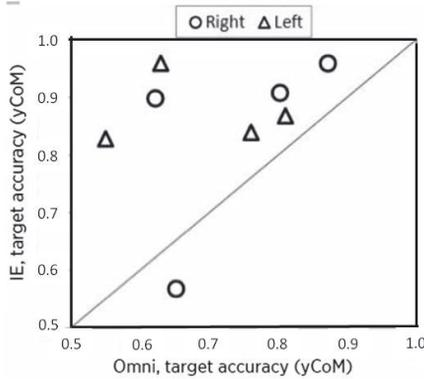
**Fig. 5:** Scatter-plot comparing individual localization performance between the Omni (x-axis) and IE (y-axis) condition for sounds arriving from the sides (left quadrant: triangles; right quadrant: circles) for the four poorest performers ( $yCoM < 0.87$ ).
