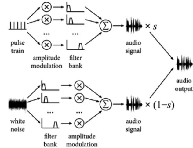
**Fig. 2:** Block diagram illustrating signal synthesis in the model of frequency perception. Two different carrier signals are combined according to the synchronization factor  $s$ .
