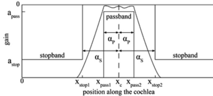
**Fig. 3:** Bandpass filter specification illustrating parameters to determine the filter bandwidth.
