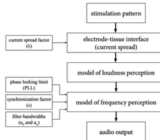
**Fig. 1:** Block diagram of the acoustic simulation algorithm. On the left-hand side simulation parameters are illustrated that can be configured to simulate different capabilities of a CI user.
