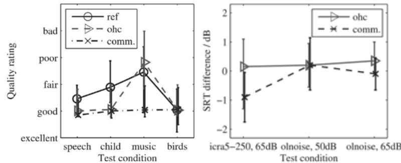
**Fig. 3:** Left: Quality rating. Right: Difference of individual speech reception thresholds (sentence test OISa) between ref and the indicated algorithm. Negative values indicate better speech intelligibility.
