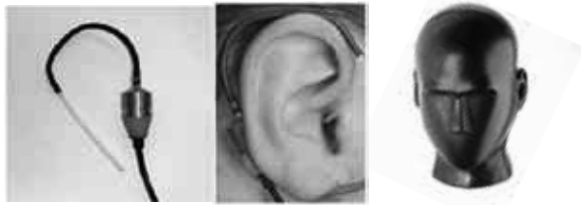
Fig. 1: Methods for measurements of binaural transfer functions; left and middle: self-made probe microphones for individual customization, right: dummy head (Neumann Ku-80) customization
