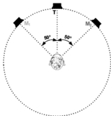
Fig. 3: Simulated spatial setup using HRTFs. Target is in front of the subject, and the two speech maskers are presented so one has an azimuth angle of +50^\circ and the other one of -50^\circ .
