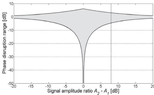
**Fig. 2:** The phase disruption range in which the sum of two harmonic signals may lie is shown by the gray area. In this plot, 0 dB corresponds to the maximum amplitude of the two signals.
