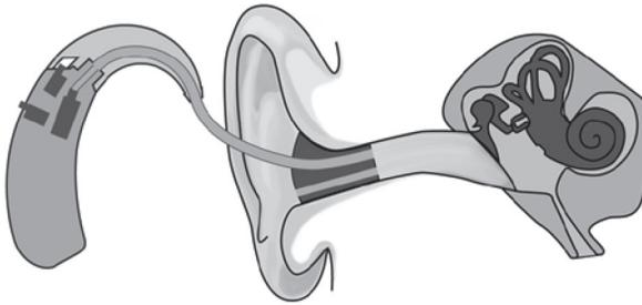
**Fig. 3:** Illustration of a ventilated in-situ HA system. The vent is connecting the residual volume to the outside.
