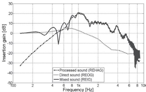
**Fig. 5:** Simulated example of the mixing of the REHAG and the REOG at the eardrum for a flat 30-dB-HL and a 3-mm $\varnothing$  cylindrical vent.
