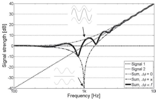
**Fig. 1:** Illustration of the phase disruption phenomenon. Inserts illustrate constructive (in-phase) and destructive (antiphase) interference.
