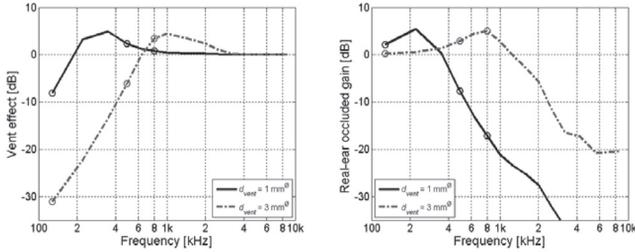
**Fig. 4:** The vent effect (left panel) and the REOG (right panel) as function of frequency exemplified for two vents with different diameters and equal lengths. Values indicated in the plots with circles at  $f=125$  Hz, 500 Hz and 800 Hz are used in Fig 6.
