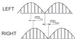
Fig. 1: Illustration of a modulated electric pulse train with ITD in the carrier (fine structure) and in the envelope.
