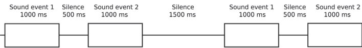
Fig. 4: Timeline presentation of one test case. The durations of sound events and silences are in milliseconds.
