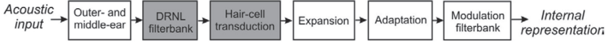
Fig. 2: Structure of the model's front-end. The acoustic input is processed by several stages of auditory processing to form an internal representation with axes; time, frequency and modulation frequency.
