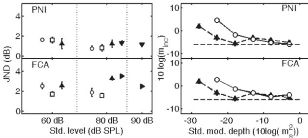
**Fig. 4:** Left panels show the data from the JND measurements. Open circles indicate JNDs with noise (20 Hz – 8 kHz), open squares (1 – 8 kHz), upward triangles tonal JNDs at 1 kHz, downward at 4 kHz and right-pointing indicate 3 kHz. Right panels show data from the modulation depth discrimination task. Closed triangles represent data from NH listeners. Open circles indicate data from HI listeners at a carrier frequency of 1 kHz.
