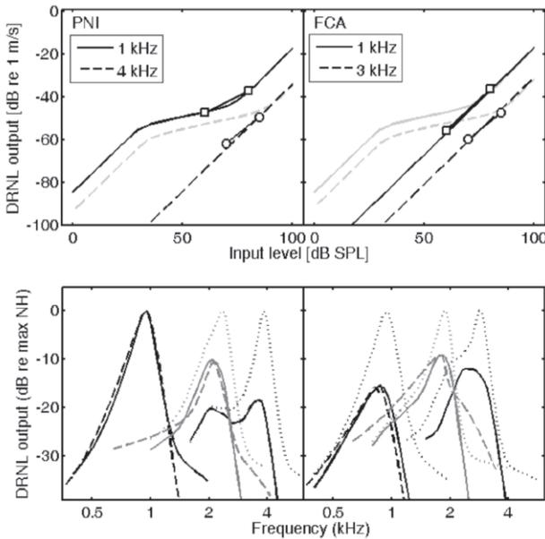
**Fig. 5:** Top panels: Input/output functions of the DRNL filter fitted to the slopes derived from the forward masking experiments (marked with symbols) Gray lines indicate the NH functions. Bottom: Iso-intensity response curves of the DRNL filter at different center frequencies. Dotted curves indicate filters for NH, solid curves indicate filters for HI listener and dashed curves indicate estimated filter shapes based on the notched-noise data.
