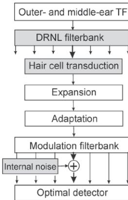
**Fig. 1:** The auditory processing model comprising stages of the outer- and middle-ear, DRNL unit, hair cell transduction, expansion, adaptation, modulation filterbank and the optimal detector.
