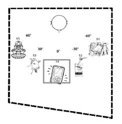
**Fig. 2**: Schematic top-down view of the simulated room, showing the virtual listener and the five sound sources at  $0^{\circ}$  (S1),  $\pm 30^{\circ}$  (S2, S3), and  $\pm 60^{\circ}$  (S4, S5). S1 (telephone sound) was moving either in the left-right or near-far direction (see text for details).
